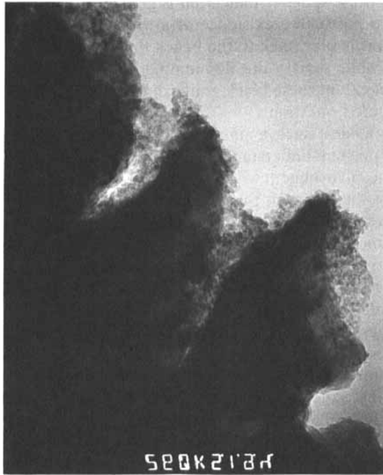
FIGURE 3 Transmission Electron Micrograph of an ultra-thin cross-cut on the boundary of rolled steel.
